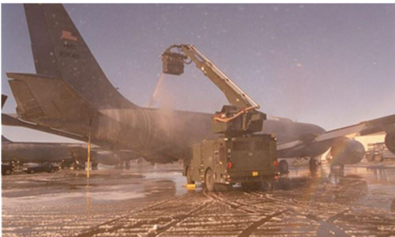
A Pease deicer does its job to free a N.H. KC-135 during a brutal cold streak at the start of 2001.
